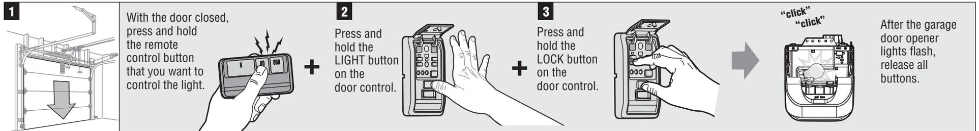
Test by pressing the remote control button. The garage door opener lights should turn on or off but the door should not move.
